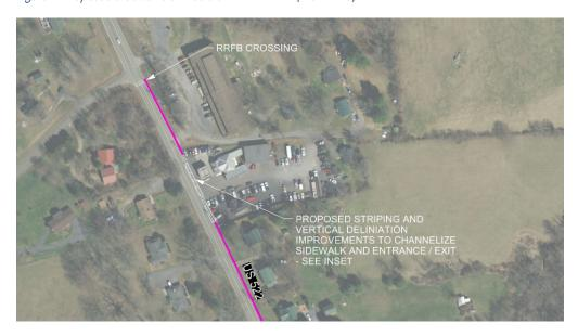
Figure 3. Proposed Striping and Vertical Delineation at Settle's Grocery and Garage in Flint Hill
